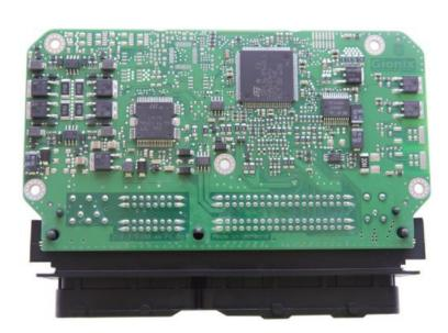
Gionix MZ series engine control units are the first and only Ukrainian ECU's that comply to European emission standards up to Euro-5 (ongoing Euro-6 certification) and delivered on conveyor of JSC "Zaporozhye Automobile Building Plant".
